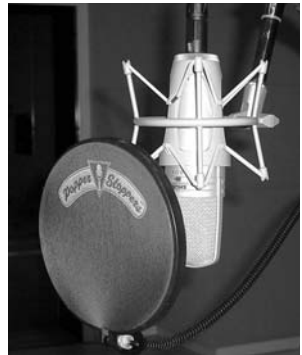
Example of a shock mount and a pop filter.
